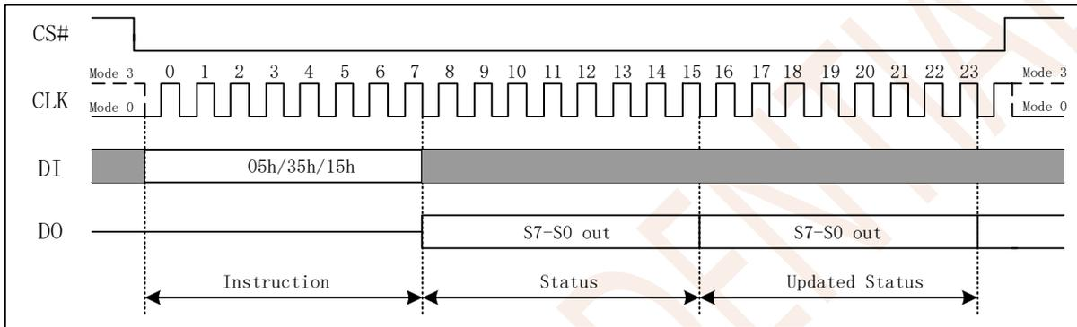
Figure 7.1a Read Status Register Instruction (SPI Mode)
