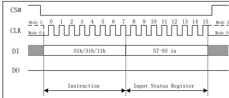
Figure 7.5a Write Status Register Instruction (SPI Mode)
