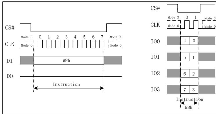
Figure 7.35 Global Block Lock Instruction(SPI or QPI Mode)
