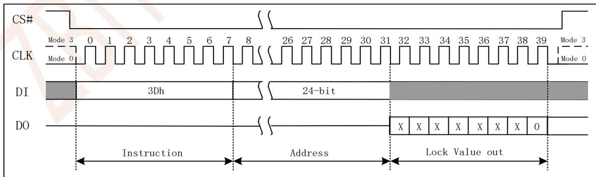
Figure 7.33a Read Block Lock Instruction (SPI Mode)
