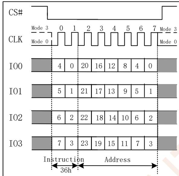
Figure 7.31b Individual Block/Sector Lock Instruction(QPI Mode)
