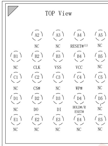
Figure 3.4 24-BALL TFBGA (5x5 ball array)
