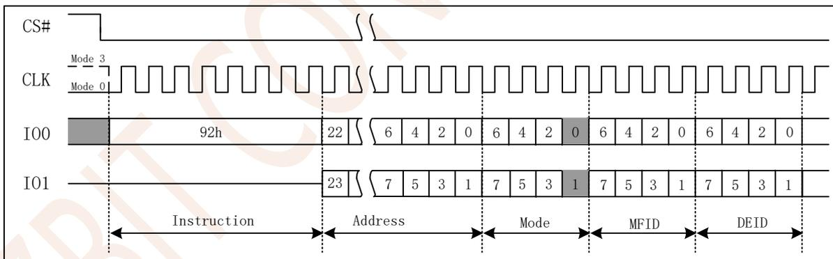
Figure 7.36 Read Manufacturer/Device ID Dual I/O Instruction
