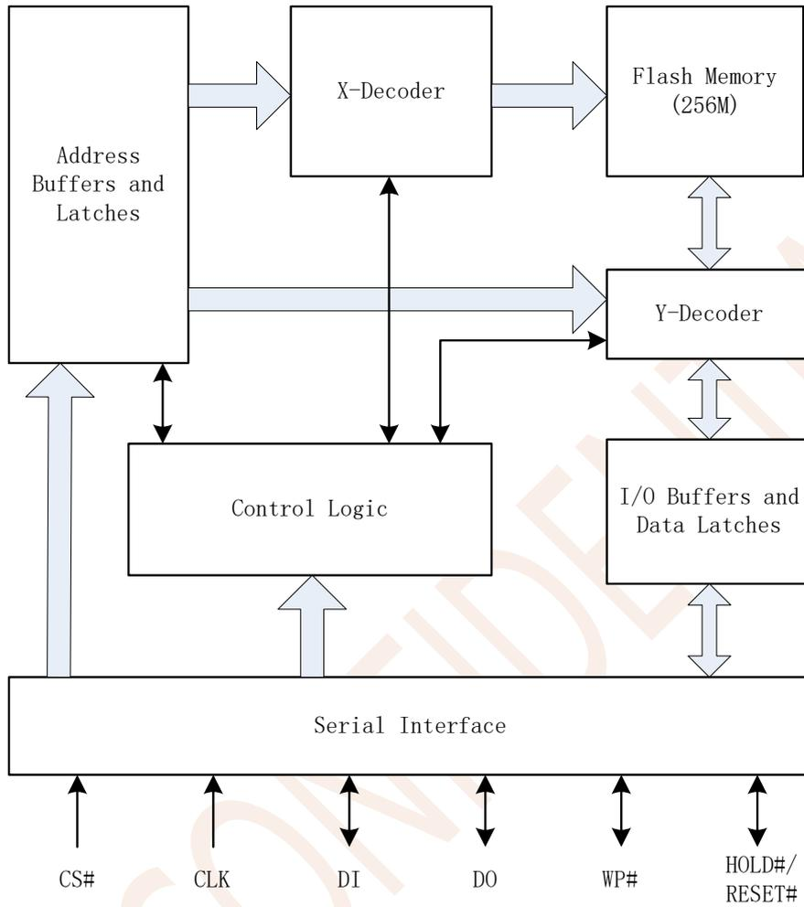
Figure 2.1 Block Diagram
