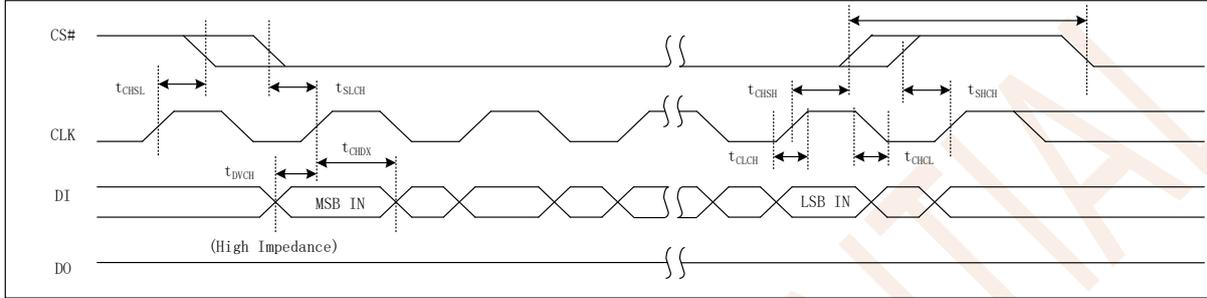
Figure 8.5 Input Timing
